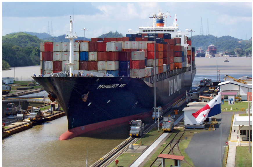
Piled up: Globalised trade has driven up both the size and the number of container ships crossing the oceans to the extent that by now many are too large to fit through the existing locks of the Panama Canal. The image shows a ship of the Panamax format, the Providence Bay, crossing the Panama Canal. (Photo: Biberbaer/Wikicommons.)
