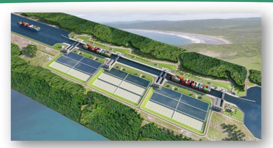
3 water saving basins per lock chamber required
